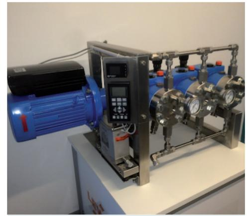
Bronkhorst's mini CORI-FLOW M15 Coriolis Mass Flow Meter in combination with LEWA's PID-controlled LDB3 three head pump.
