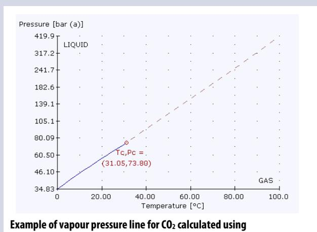
Example of vapour pressure line for CO<sub>2</sub> calculated using
