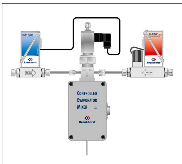
Single carrier gas supply, no dilution, thermal liquid flow meter
